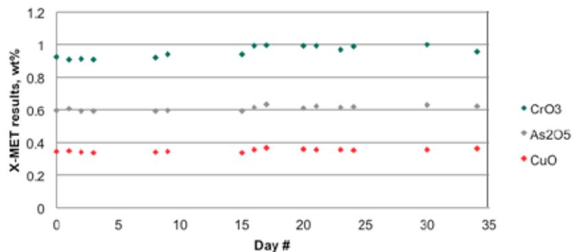
Note: The X-MET8000 offers total versatility. For example, wood preservative solutions can also be analysed. To do this, users can create their own calibrations by measuring a set of calibration standards (solutions with known elements' concentrations). Calibrations can also be added by our Applications Support teams on request.
