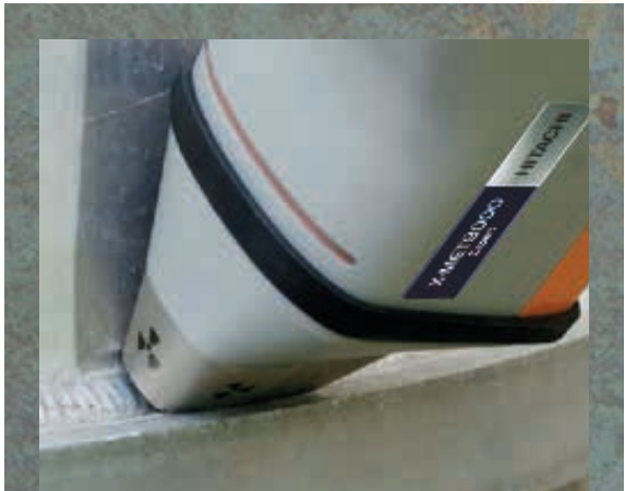
Analysis of small, hard-to-reach areas with the X-MET8000
