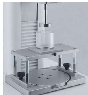
TX-ECF : EXTRUSION CELL FIXTURE (Ref. 100200)
