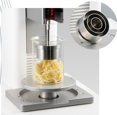
TX-TRPF : THREE RINGS PROBE CUTTING FIXTURE (Ref. 130186)
