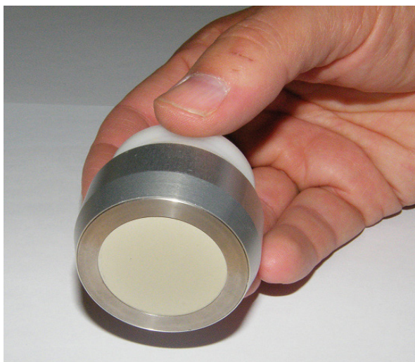
Pressed pellet in pellet holder
