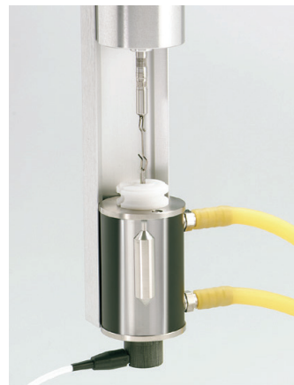
Standard Sample Chamber with embedded temperature probe provides direct temperature measurement of sample
