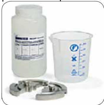
Figure 3: Calibration Test Kit with Viscosity Standard Fluid
