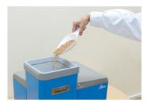
Fill the grain into the shaft of InfraLUM FT-12 WholeGrain, choose the analyzed product in the menu and start the measurement.
