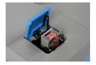
Put the cell into the InfraLUM FT-12 analyzer, choose the analyzed product in the menu, and start the measurement
